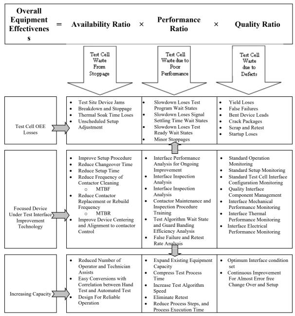
**Conclusion:** Improving OEE can happen in a number of ways. As OEE is a pice of TPM, the approach taken in this paper is to connect OEE loses, and TPM waste as a systemic approach for increasing OEE. So far, we have identified 2 types of waste and test cell loses.
